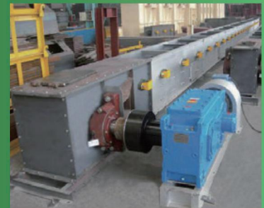
Buried scraper chain conveyor
