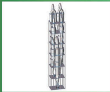
Five-stage cyclone preheater
