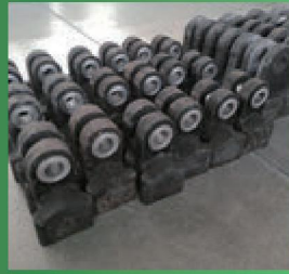
Grate cooler hammer
